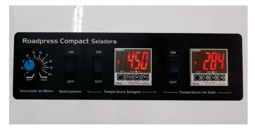
DC drive with ajustable velocity Cooling zone switch (garantees a perfect seal finish) PID Digital autotune temperature control for sealing bars PID Digital autotune temperature control for ink coder
