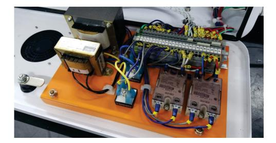
Easy access for electrical maintenance Labeled wire conectors simplifyes everything Solid state relays controls the power (400W of sealing)
